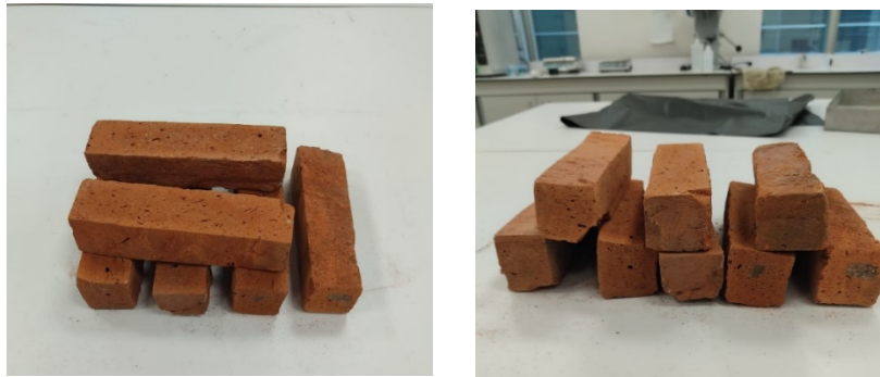
Figure 2. Produced geopolymer brick samples
