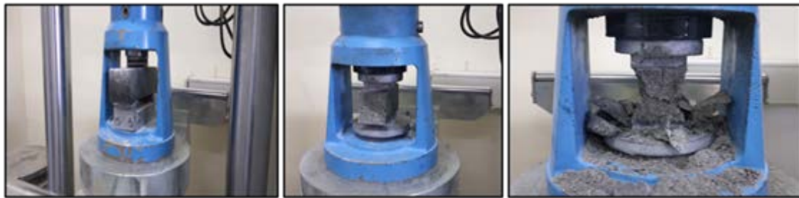
Figure 13. Bending and Compressive Strength Tests on Beam Samples
