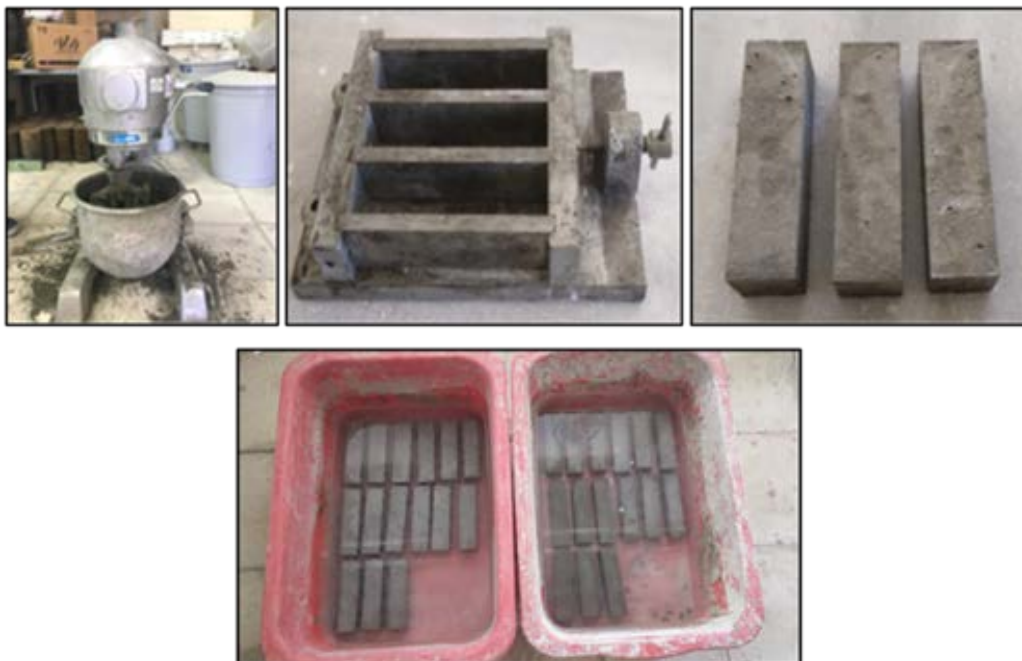
Figure 12. Preparation of Prism Samples used in Flexural and Compressive Strength tests, curing of molds and samples removed from molds
