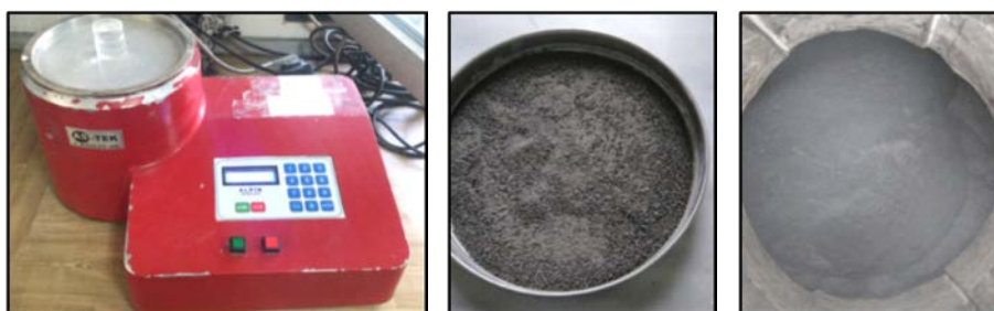
Figure 3. Sieve device used in dimensional analysis
