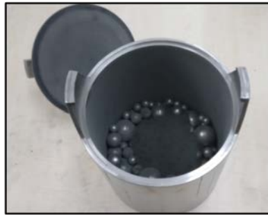
Figure 5. Grinding Bowl and Grinding Ball Surfaces
