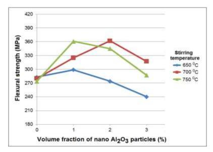
**Figure 7.** The flexural strength of ENAC-46000 Al alloy and Al-Al<sub>2</sub>O<sub>3</sub> composites depending on stirring temperature at 300 rpm
