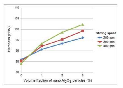
Figure 4. The hardness of ENAC-46000 Al alloy and Al-Al<sub>2</sub>O<sub>3</sub> composites
