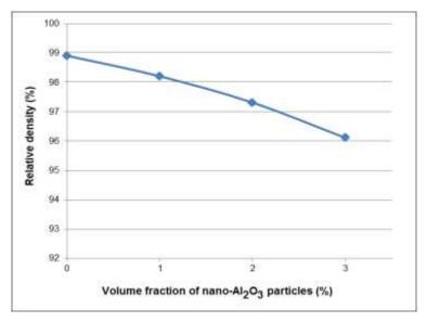
Figure 3. Relative densities of ENAC-46000 Al alloy and Al-Al<sub>2</sub>O<sub>3</sub> composites manufactured at 700  $^{0}$ C and 300 rpm
