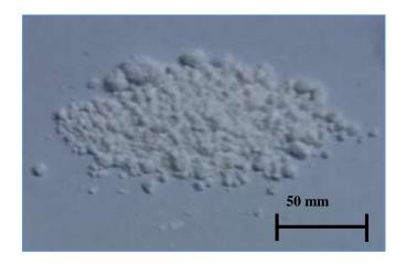
Figure 1. Agglomerated nano Al<sub>2</sub>O<sub>3</sub> reinforcement particles
