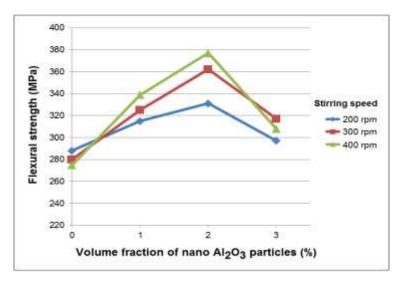
Figure 6. The flexural strength of ENAC-46000 Al alloy and Al-Al<sub>2</sub>O<sub>3</sub> composites depending on stirring speed at 700  $^{0}$ C
