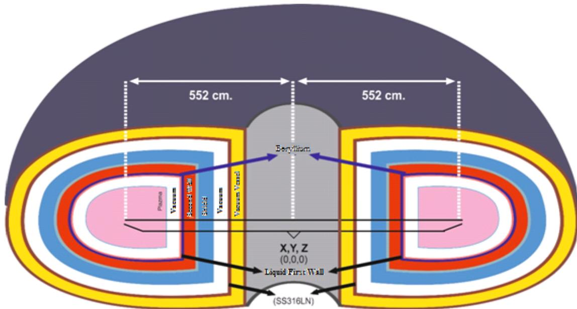
**Figure 1.** Representation of the APEX hybrid reactor used in calculations.
