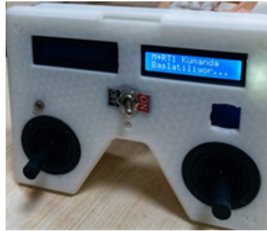
Figure 5. The designed wireless controller.
