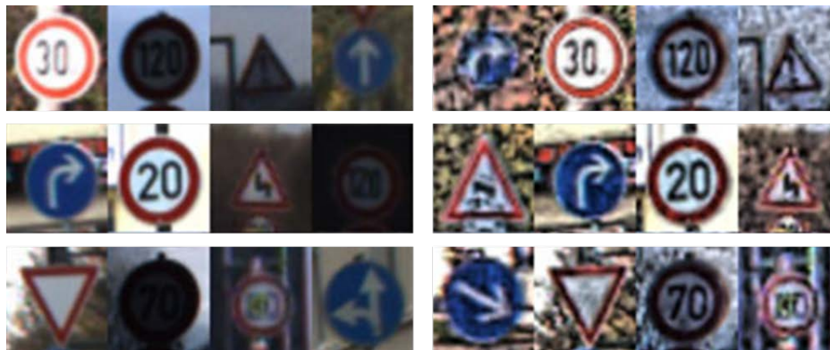
Figure 7. Preprocessed samples of images with the CLAHE algorithm
