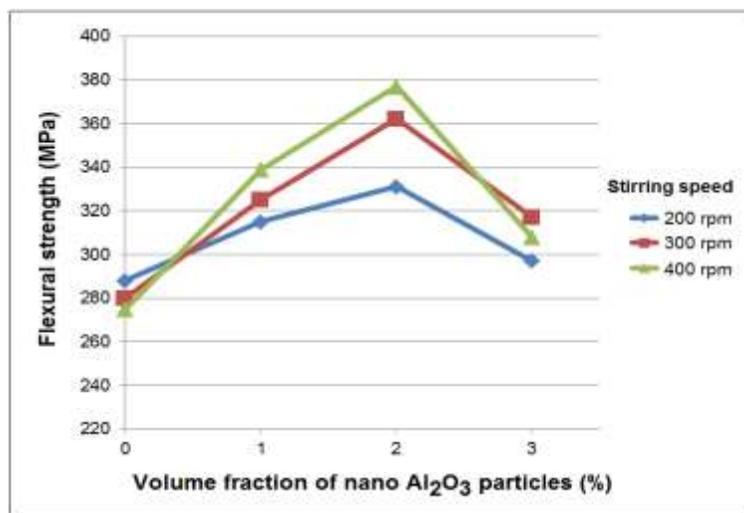
**Figure 6.** The flexural strength of ENAC-46000 Al alloy and Al-Al<sub>2</sub>O<sub>3</sub> composites depending on stirring speed at 700 °C
