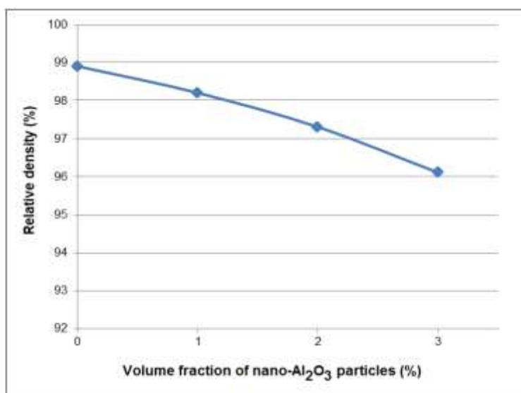
**Figure 3.** Relative densities of ENAC-46000 Al alloy and Al-Al<sub>2</sub>O<sub>3</sub> composites manufactured at 700 °C and 300 rpm
