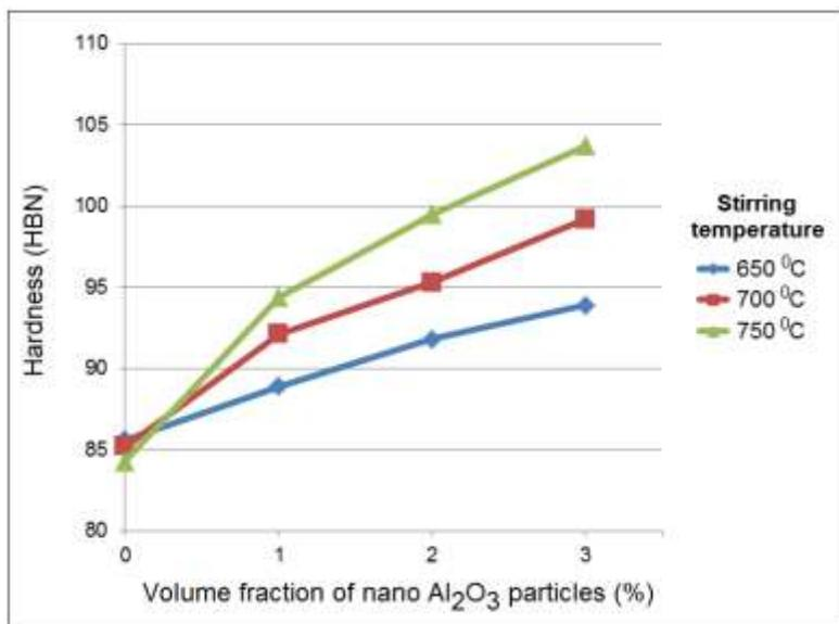
**Figure 5.** The hardness of ENAC-46000 Al alloy and Al-Al<sub>2</sub>O<sub>3</sub> composites depending on stirring temperature at 300 rpm
