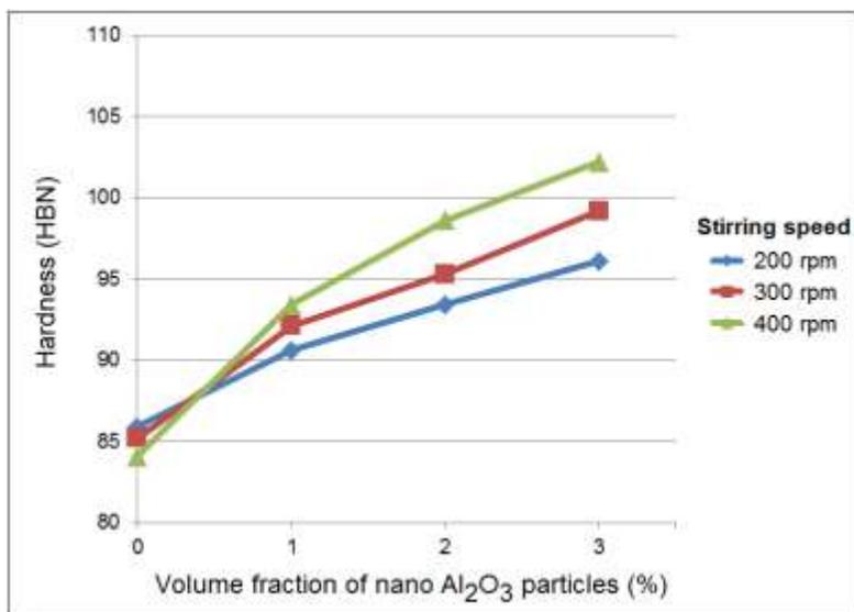
**Figure 4.** The hardness of ENAC-46000 Al alloy and Al-Al<sub>2</sub>O<sub>3</sub> composites depending on stirring speed at 700 °C
