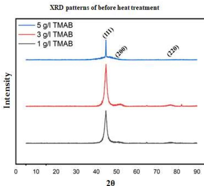
**Figure 1.** XRD patterns of the as-deposited coatings containing: 1 g/L, 3 g/L and 5 g/L boron.
