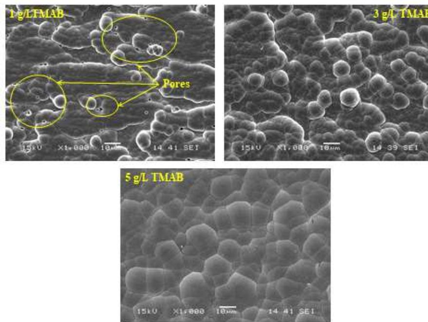
**Figure 4.** SEM micrographs of surface morphology of Ni-B coatings: 1 g/L, 3g/L and 5 g/L, respectively.
