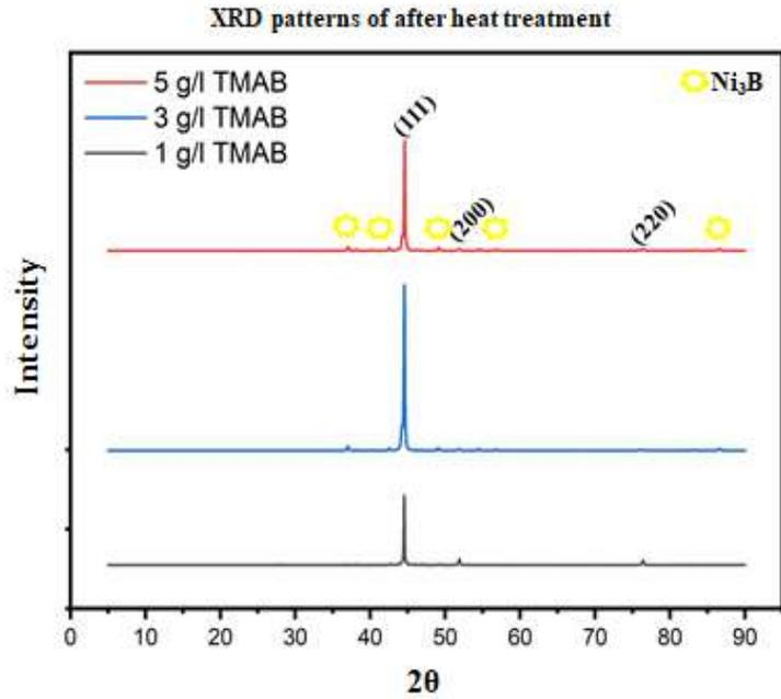
**Figure 2.** XRD patterns of heat treated coatings containing: 1 g/L, 3 g/L and 5 g/L boron.
