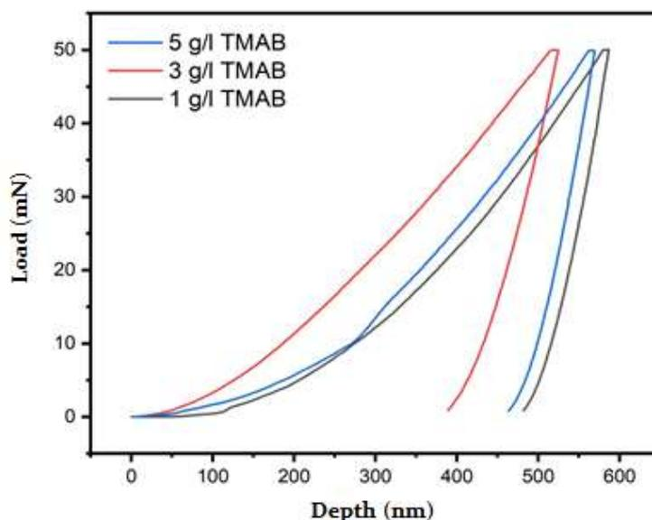
**Figure 7.** Load-depth curves for 1 g/L, 3 g/L and 5 g/L.
