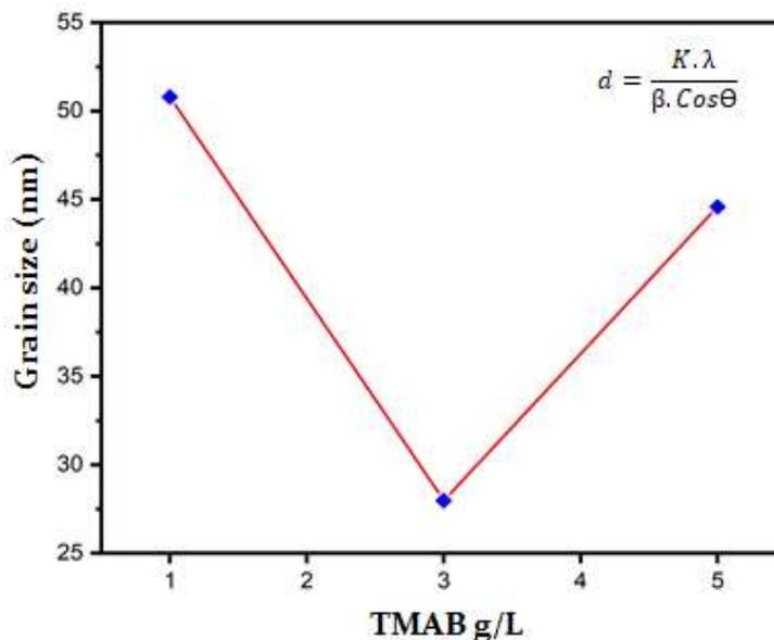
**Figure 3.** Changes in the crystalline size of heat treated coatings as a function of the amount of TMAB.
