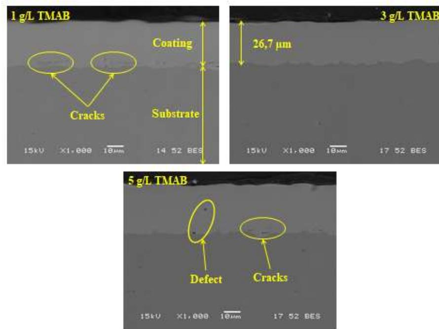
**Figure 5.** Cross-sectional SEM images of coatings.
