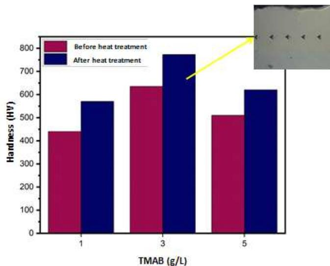
**Figure 6.** Hardness change of Ni-B coatings as a function of pre-heat and post-heat treatment temperature.
